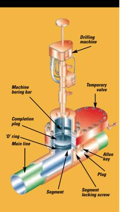
Following the line plugging process, the drilling machine can be used once again to lower the completion plug through the valve and into its final position. Segment locking screws secure the plug while the boring bar is retracted. The drilling machine is then removed, followed by the temporary valve, and a flange fitted over the completion plug to complete the seal.
