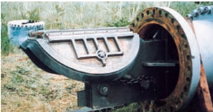
48" (1200mm) folding head for crude oil line stop.
