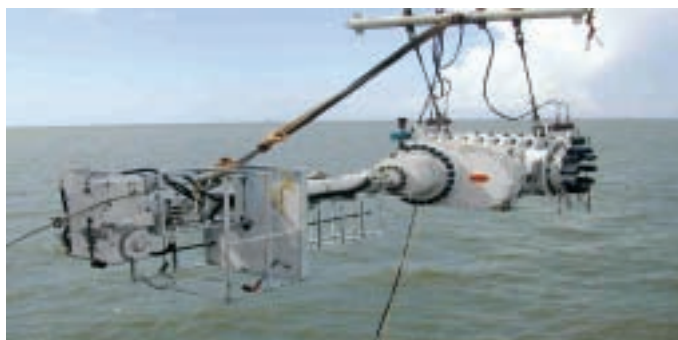
914XL hot tap machine with hot tap fitting.
