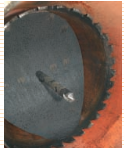
36" hot tap cutter, coupon and pilot drill.
